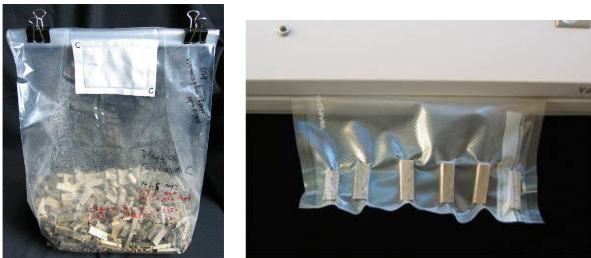
Figure 1. Ophiostoma clavigerum growing on inoculated wood pieces with vermiculite in a patch bag (left), vacuum sealing (right).
