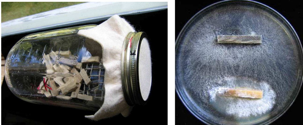
Figure 3. Air-drying of samples placed on stainless steel mesh inside Mason® jar that is closed with metal ring and a piece of sterile cotton flannel fabric (left). Fungi growing out of air-dried naturally infested material at the time of assessment (right).
