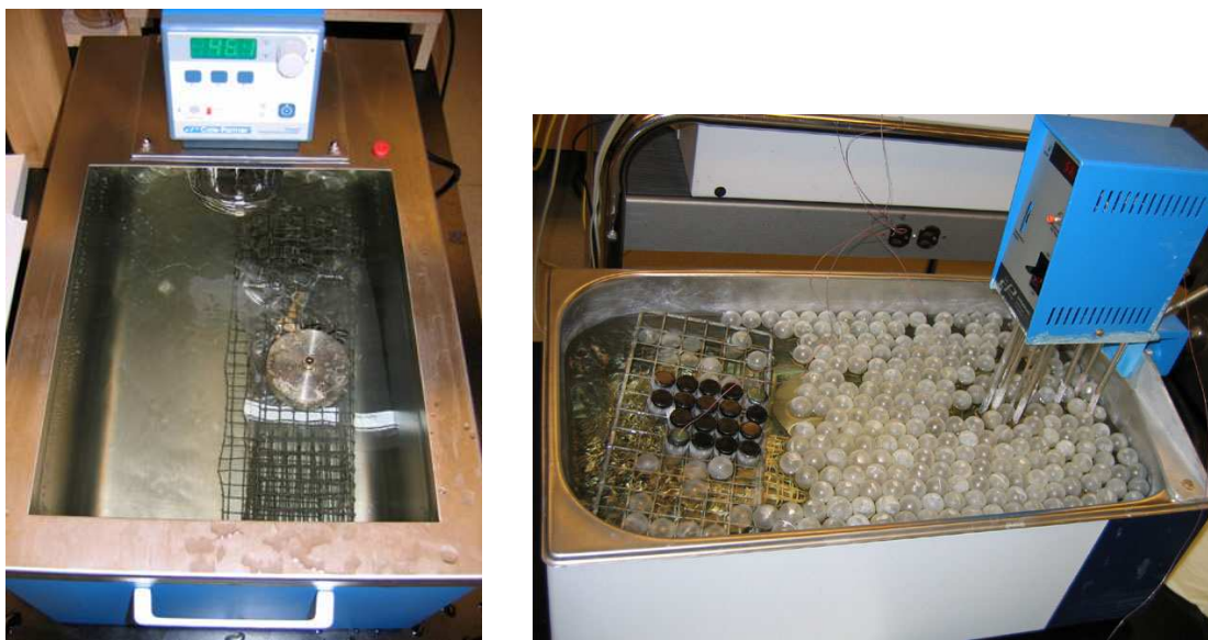
Figure 2. Water bath equipped with Polystat® temperature controller, heated at target temperature, test wood enclosed in vacuum-sealed bag and sandwiched together between two mesh grids is being held on the bottom of water bath (left). Heat treatment of fungi grown in vials held in vial racks with the lids remaining above the water line (right).
